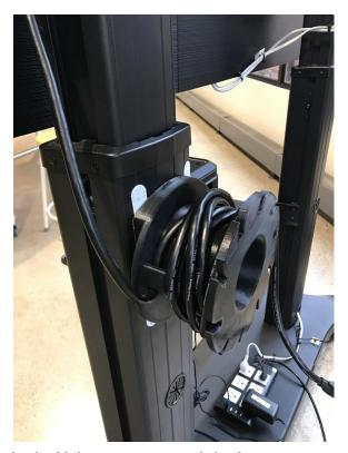
In the Makerspace, we used the Structure Sensor to reverse engineer the curvature of our TV stand. We then 3D printed a case that fits snugly and holds the HDMI cord.
