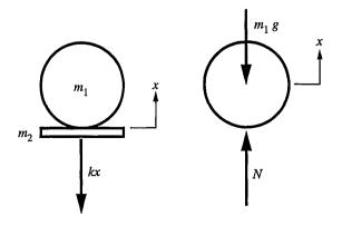
We consider the system to move away from its static equilibrium position a distance x upward, which serves as the generalized coordinate. Hence, the spring force acts downward. The gravity force has a static effect, which is irrelevant to the equation of motion because x is measured relative the static equilibrium position. Hence, the equation of motion resulting from the first free body diagram is
