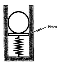
This exercise is intended to bring out the way in which static and dynamic forces might occur in a study, as well as to highlight interpretation of harmonic response. We begin by drawing two free body diagrams. The first, which we will use to derive the equation of motion, considers the sphere and the platform as a system, so that the contact force exerted between these bodies is an internal force that is not considered.
